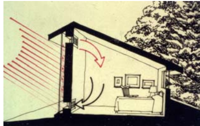
Figure A-2. Indirect Solar Gain
