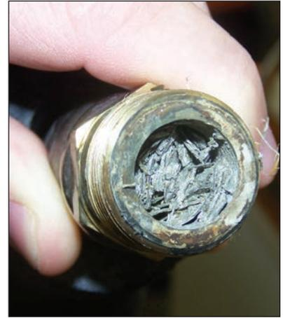
**Figure 6:** Results of failure to maintain water chemistry in two steel pipe building loops.
