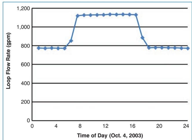
**Figure 7:** Flow rate with two-way valves interlocked with fans rather than compressors.
