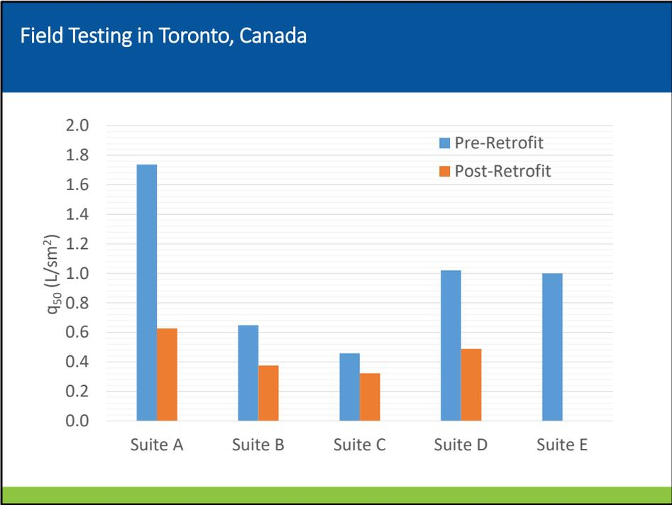
Here is an example of how the area normalized air leakage test data may be presented. This is a building that underwent an energy retrofit where there the windows were replaced and the envelope was overclad with exterior insulation – both of which improved the suite-level air tightness. However these are results of the whole suite test which includes both the interior partition walls and the exterior walls.
