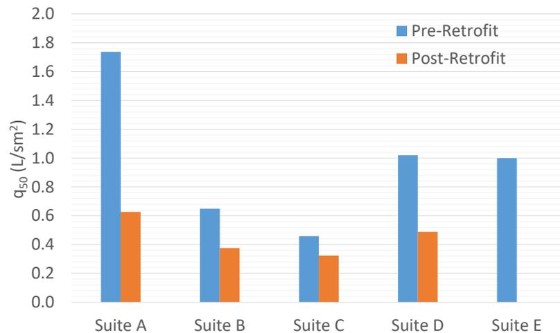
Here is an example of how the area normalized air leakage test data may be presented. This is a building that underwent an energy retrofit where there the windows were replaced and the envelope was overclad with exterior insulation – both of which improved the suite-level air tightness. However these are results of the whole suite test which includes both the interior partition walls and the exterior walls.
