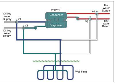
**Figure 5:** Geothermal system for simultaneous heating and cooling, operating in heating-only mode.
