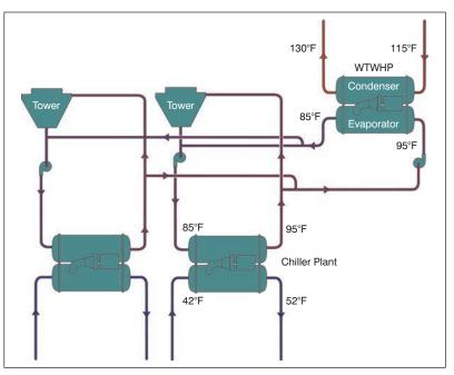
Figure 4: Tower water as heat source.
