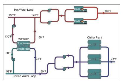
Figure 6: Side-stream arrangement.
