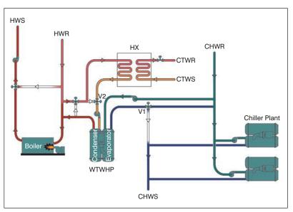
**Figure 7:** Hybrid side-stream/parallel system, operating in side-stream arrangement.
