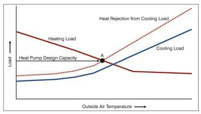
Figure 1: Selection point for simultaneous heating-and-cooling heat pump.
