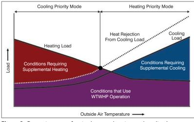
Figure 2: Operating areas for simultaneous heating-and-cooling heat pump.
