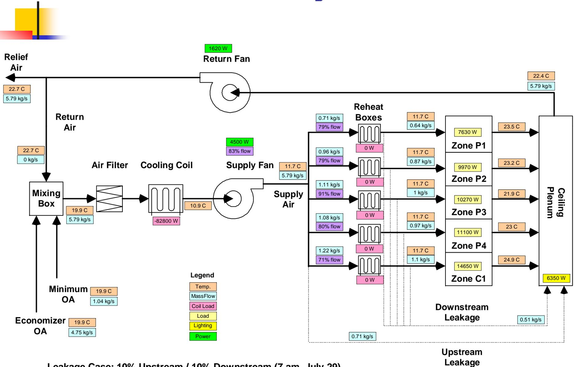
Leakage Case: 10% Upstream / 10% Downstream (7 am, July 29)
