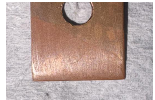
Sample coupon after coulometric reduction
