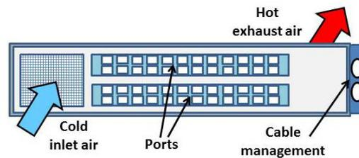
Cool air enters through the left front side of the chassis and then travels horizontally along the cards until it is directed out the right rear side.
