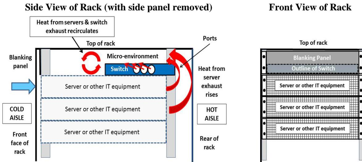
Note how the blanking panel creates a closed micro-environment within a small space that is cut off from the cold aisle where the air temperature is determined by re-circulated hot air from the server and switch exhausts. In this installation configuration, the pre-heated air inside the micro-environment is what the switch must use for its cooling.
