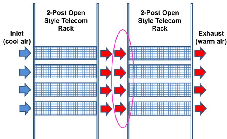
The side to side cooling air flow design of the equipment causes the warm exhaust from one piece of equipment to feed into the inlet for the cool air stream of the equipment in the adjacent rack. This installation will cause the second piece of equipment to operate at much higher inlet temperatures than intended.
