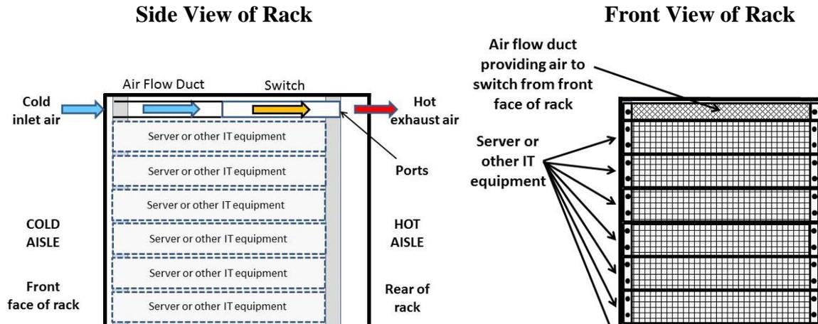
This can be achieved by a combination of a switch that has front to rear air flow and duct work that extends the switch to the front face of the rack.
