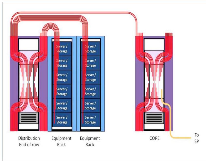
Figure 3 shows a slightly more complicated network implementation in which a distribution level has been added to the network in the form of an end of row network cabinet. The distribution equipment offloads the core equipment in both throughput and port count. In a medium to large size data center with multiple equipment rows it is common for all of the distribution networking equipment to be connected together on the same level of hierarchy to form a mesh (not shown).
