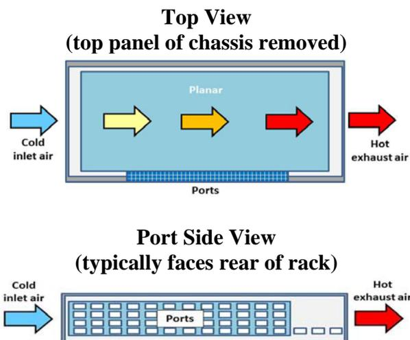
**Fig. 7E** Small 1 or 2U switch with front to rear air flow.
