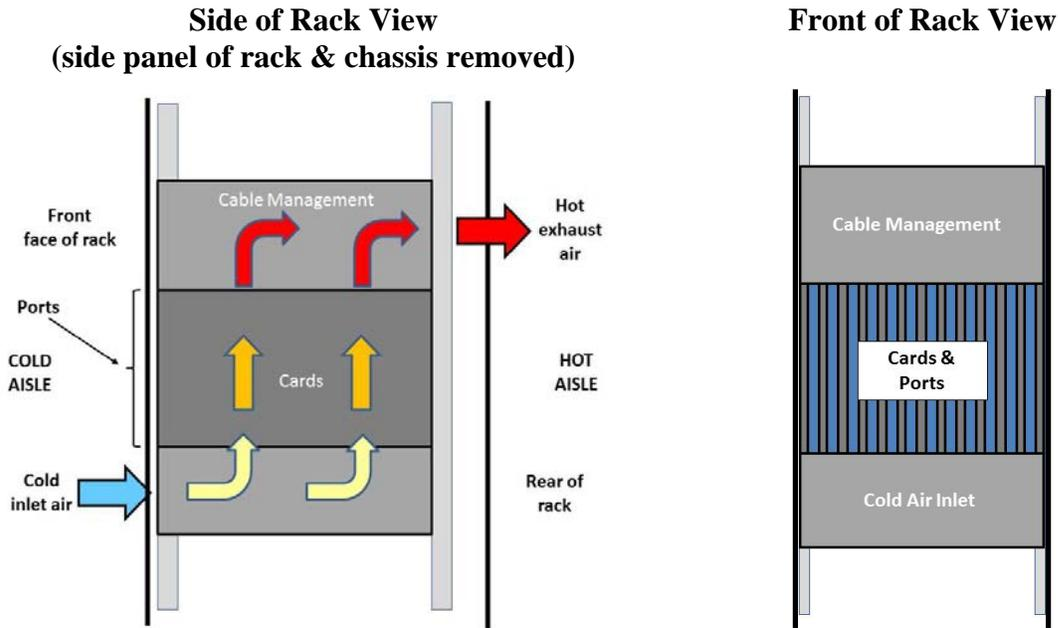
Note that the air flow is actually “S” shaped - cool air enters horizontally at the bottom front of the chassis and then travels vertically along the cards before travelling horizontally as it exits towards the rear at the top of the chassis. The network ports come off of the front facing edge of the cards and are located in the front middle of the system.
