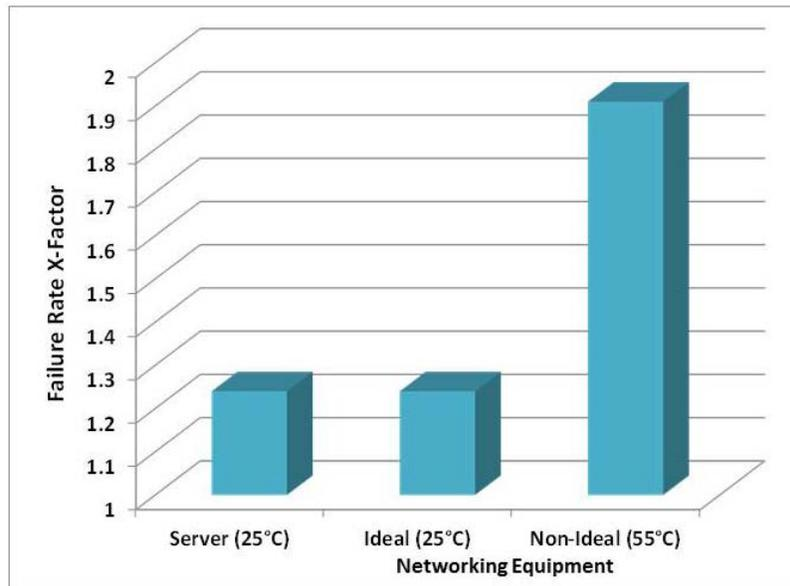
The y-axis of the plot is IT equipment failure rate relative to a 20°C air inlet temperature. The ideal and non-ideal designs are networking equipment and the non-ideal design x-factor is a top of rack switch behind a blanking panel.
