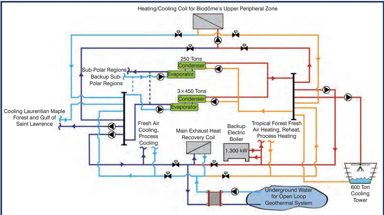
**Figure 2:** The Biodôme uses one of the largest open-loop ground-source heat pump systems in Canada.
