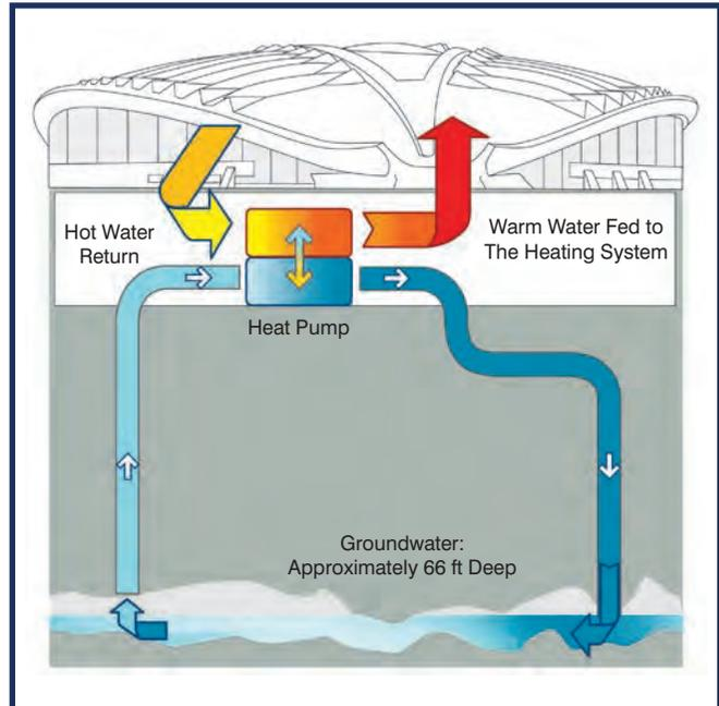
**Figure 1:** Groundwater is used for heating and cooling. In winter, the groundwater's heat is used for heating the building. In summer, excess heat from the building is transferred to the groundwater (winter mode).
