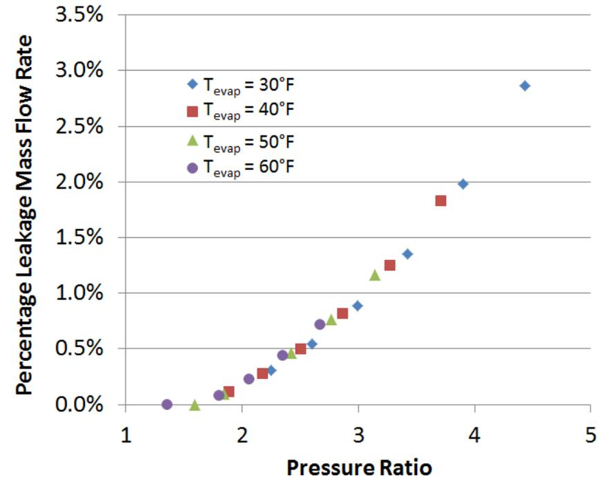
Model reveals trends in seal leakage flow rates that impact volumetric efficiency
