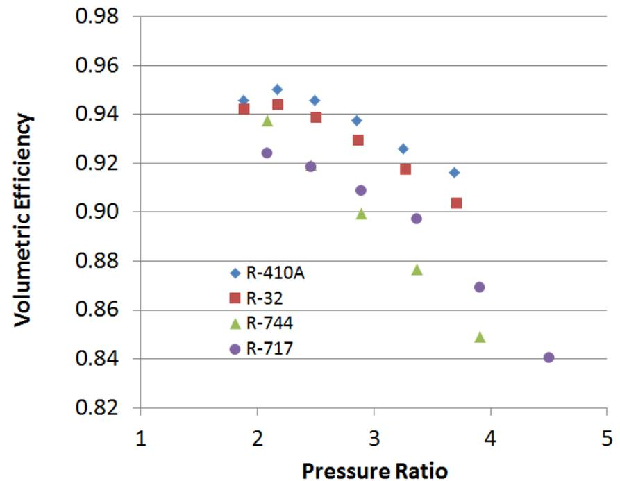
Impact of working fluid on mass flow rate and volumetric efficiency while holding evaporating temperature at 40 °F.
