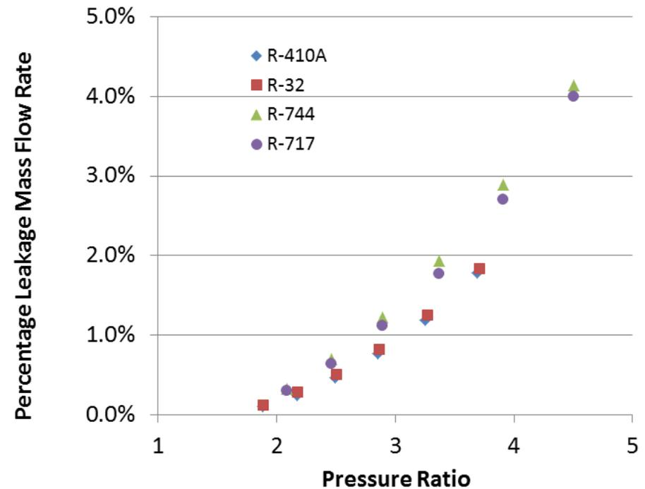
Impact of working fluid on face seal leakage flow rate while holding evaporating temperature constant at 40 °F.
