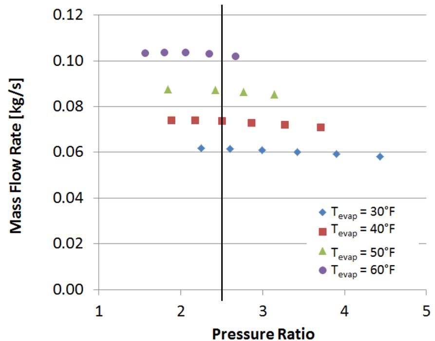
Model can predict trends in discharge temperature and mass flow rate over a range of operating conditions.
