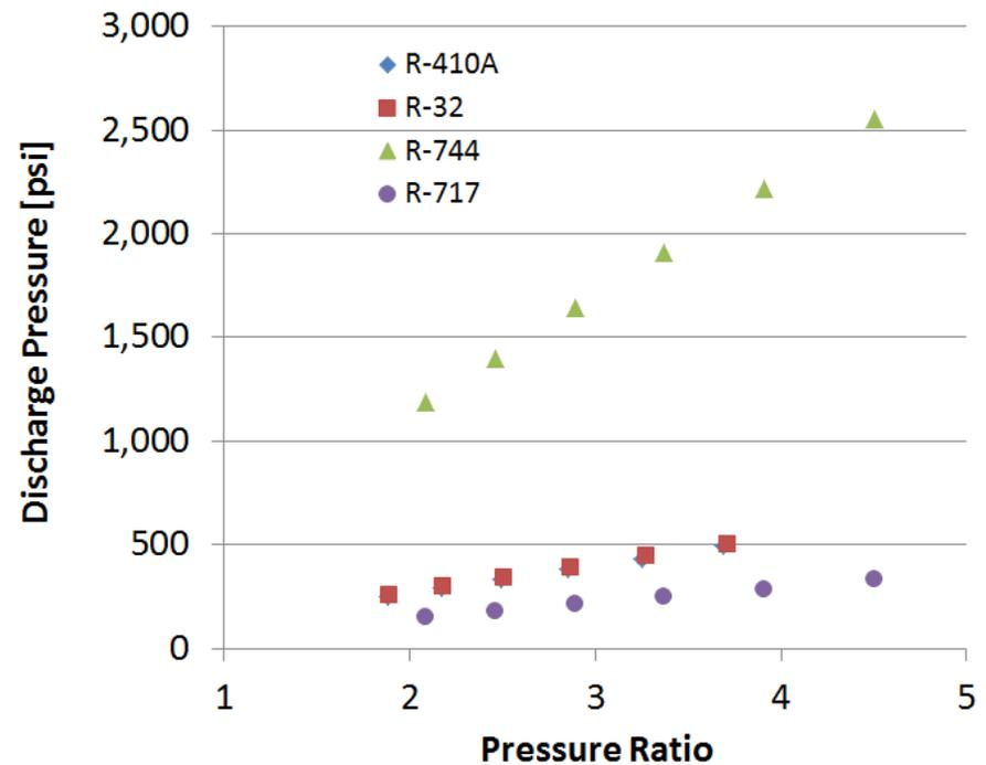
Impact of working fluid on discharge conditions while holding evaporating temperature constant at 40 °F.
