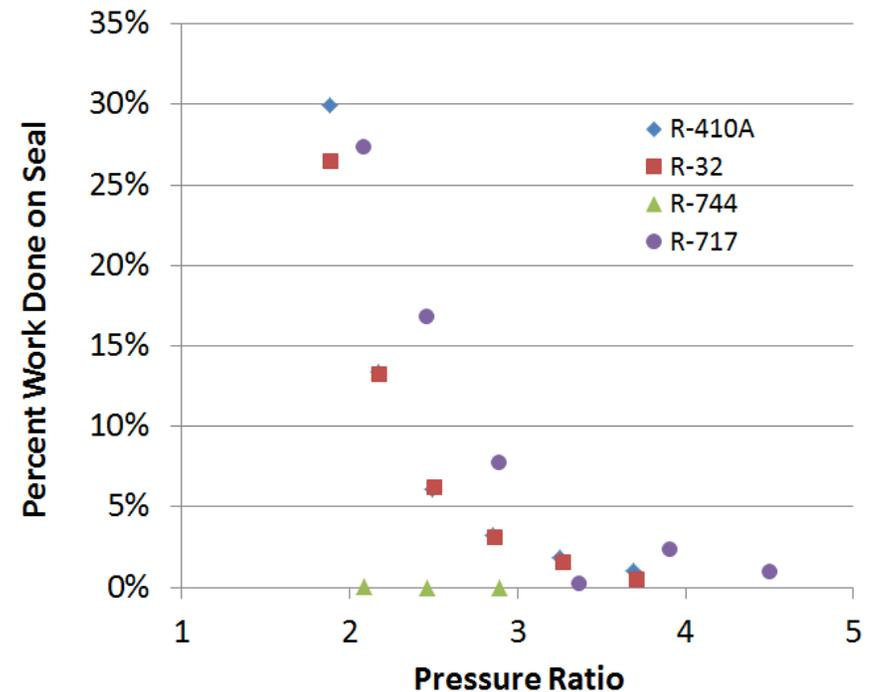
Impact of working fluid on isentropic efficiency and seal friction while holding evaporating temperature at 40°F.
