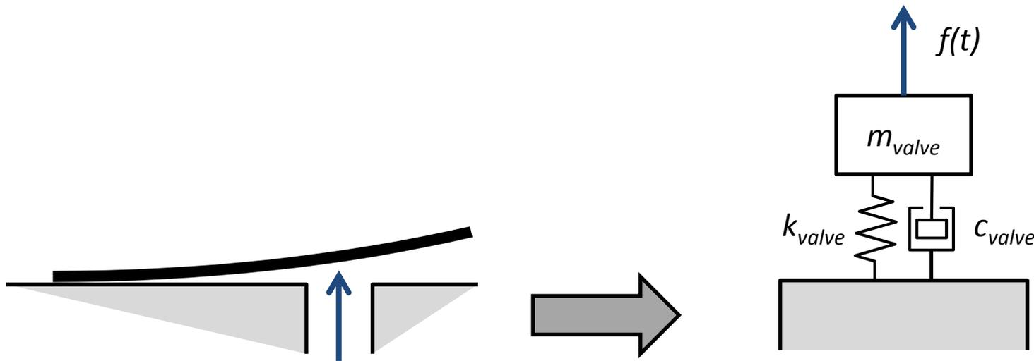
$$m_{valve}\ddot{x}(t) + c_{valve}\dot{x}(t) + k_{valve}x(t) = f(t)$$
