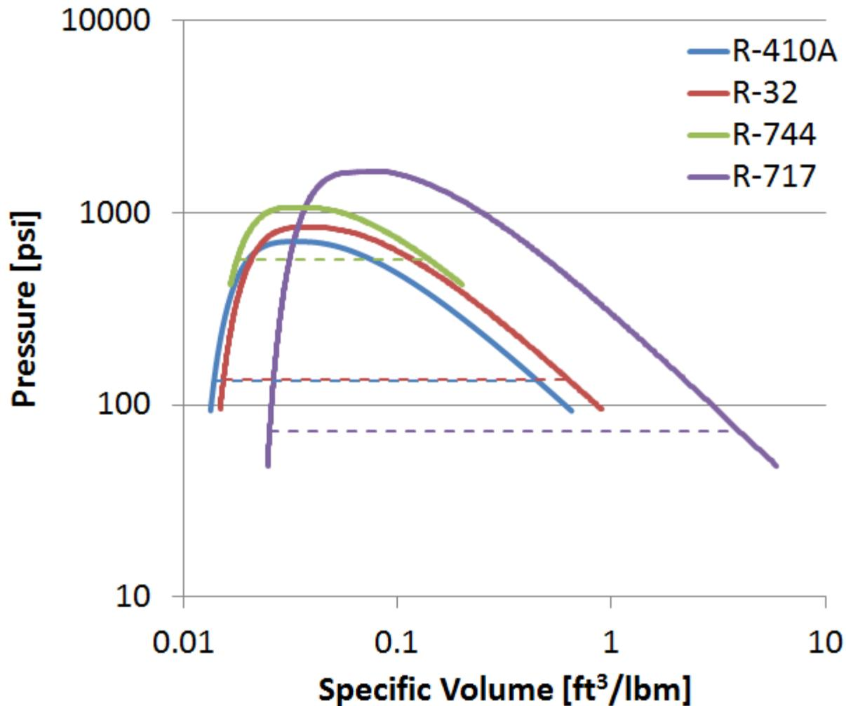
Dashed lines show saturated liquid-vapor mixture properties at 40°F.
