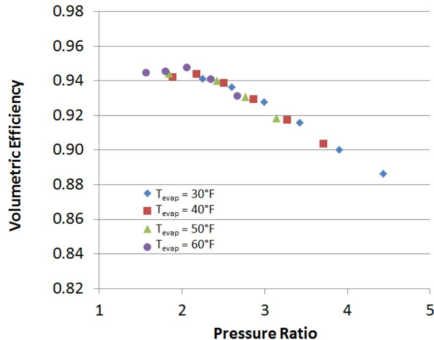
Model can predict trends in volumetric efficiency over a range of operating conditions.
