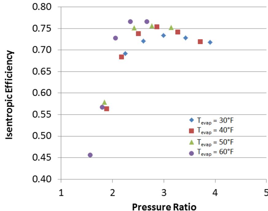
Model can predict optimal pressure ratio for maximizing isentropic efficiency
