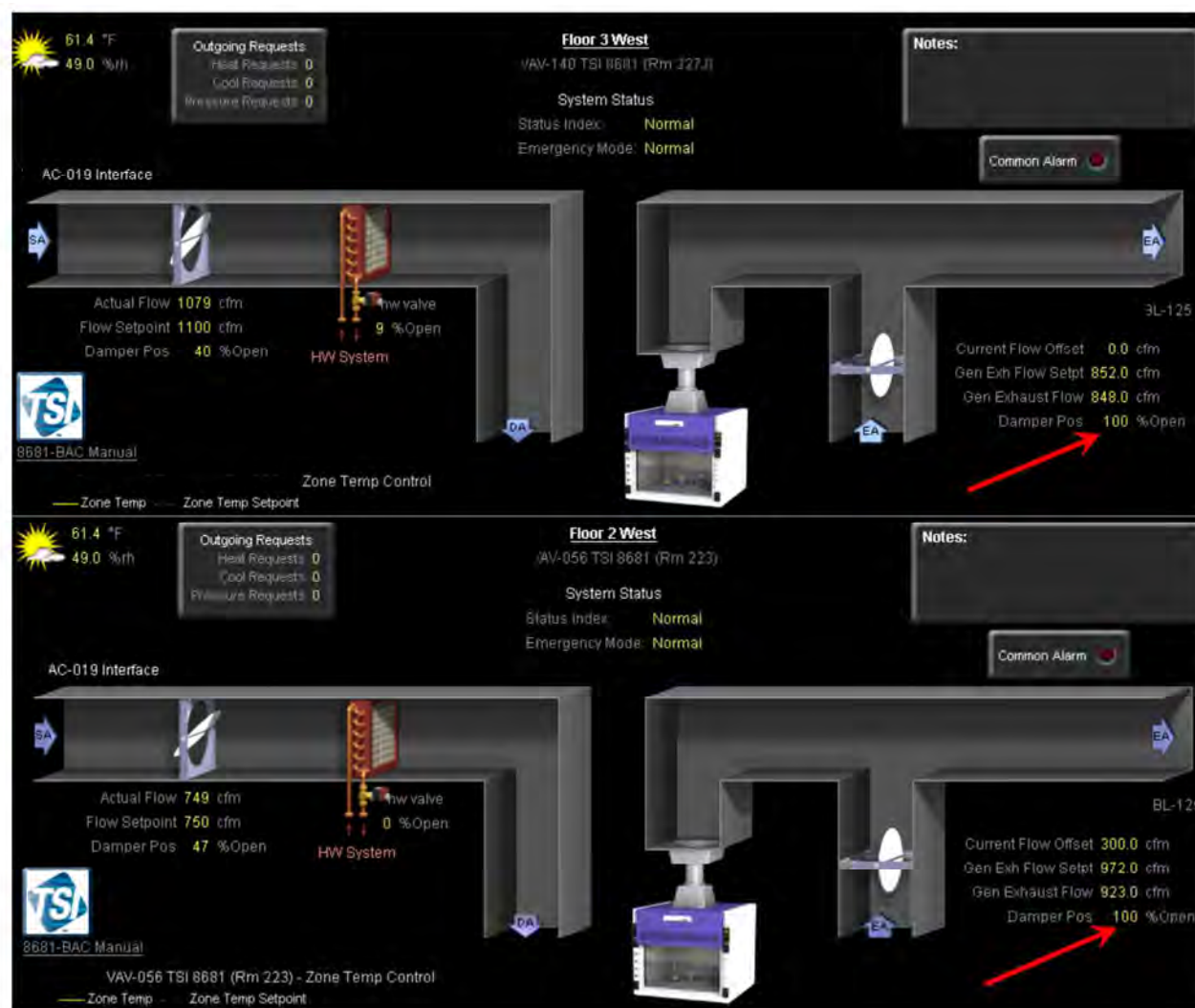
Figure 53: Exhaust dampers in 327J and 223 both starved - 100% open and slightly short of setpoint, at 1.3" exhaust plenum pressure setpoint
