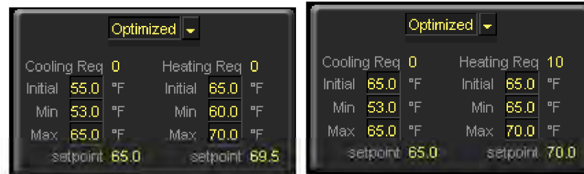
Figure 7: Original (Left) and revised (Right) supply air temperature optimization mechanism. The revised selection will operate much more smoothly because jumps in temperatures are avoided when switching from heating to cooling
