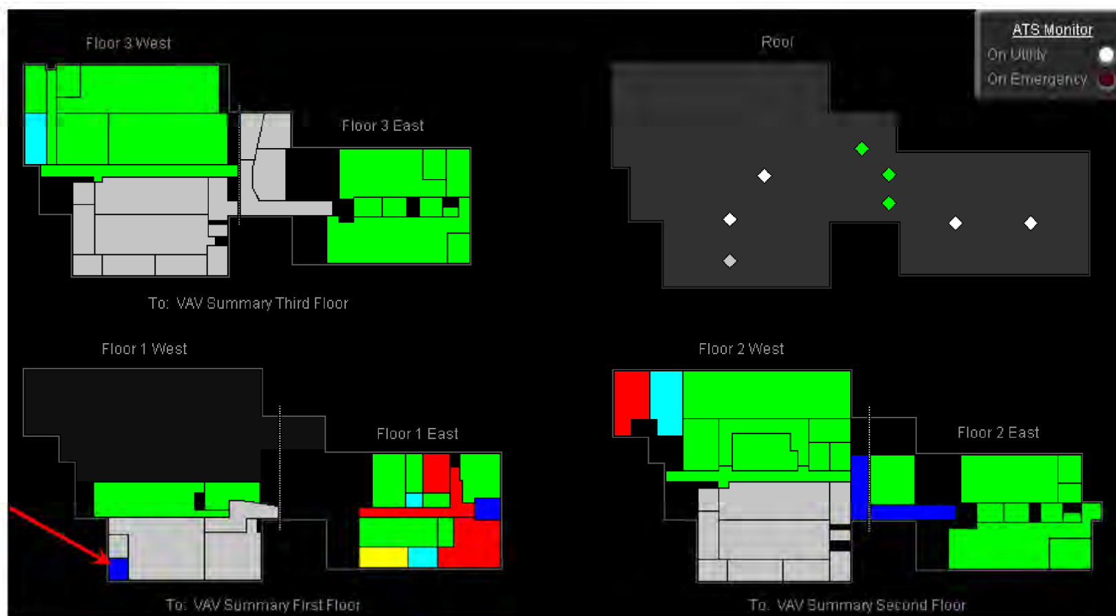
Figure 28: Override effective heat setpoint of zone 005 to 73°F to force it to “wake up” and go into setback mode. Result is blue zone on floor plan, and AC-20 re-enabled.
