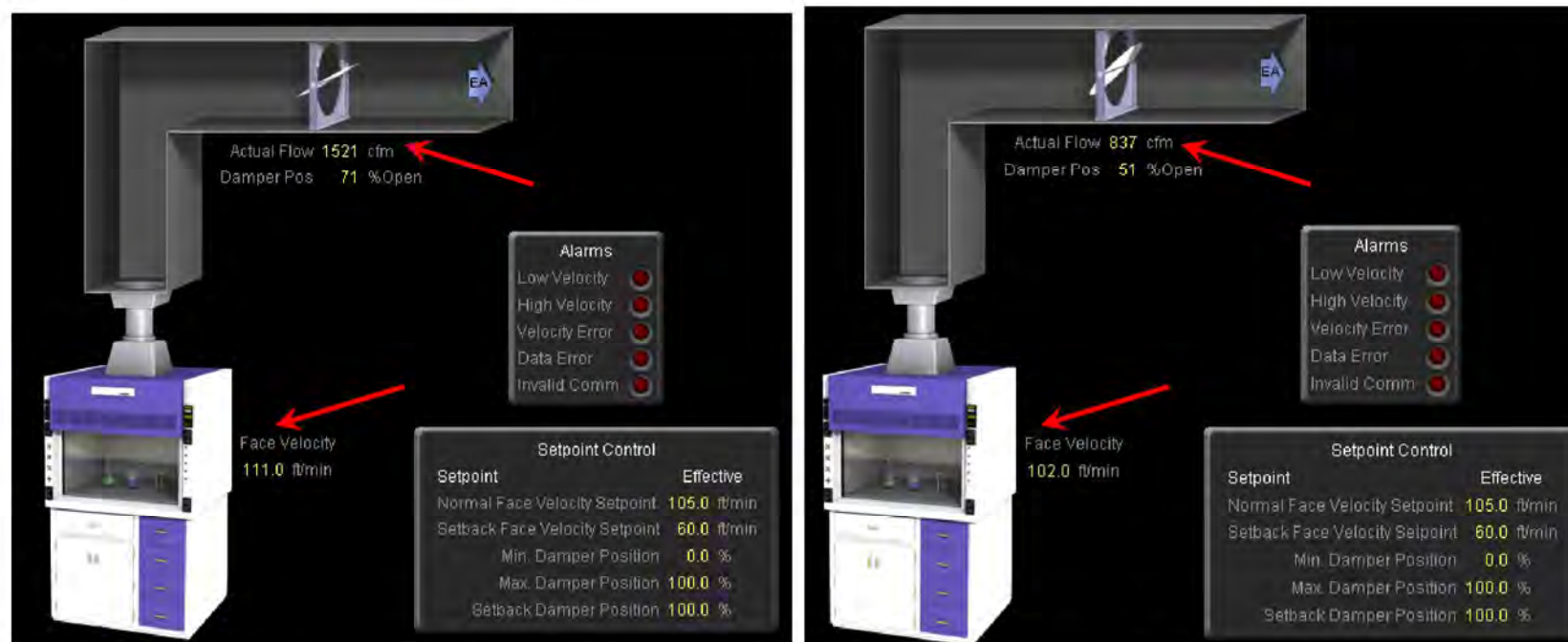
Figure 45: Temperature test, [REDACTED] 12 at 3:09PM terminals for hoods in 320B report very different airflows at sash max. position for both hoods and face velocities of 111 fpm vs 102 fpm
