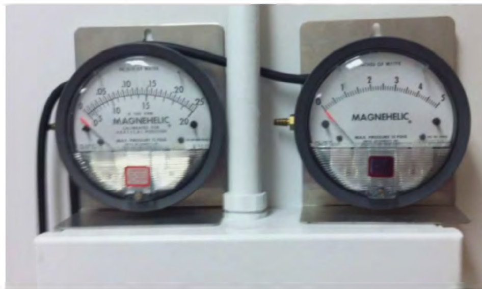
Figure 84: 2013- Measurement setup at double doors to corridor at Labs 214 and 320. Initial setup with single gauge (left), then ultimate test setup with dual gauges (for 0-0.25" and 0-5" ranges simultaneously) at right. Both rooms set up similarly before commencing first test at 8:50AM.
