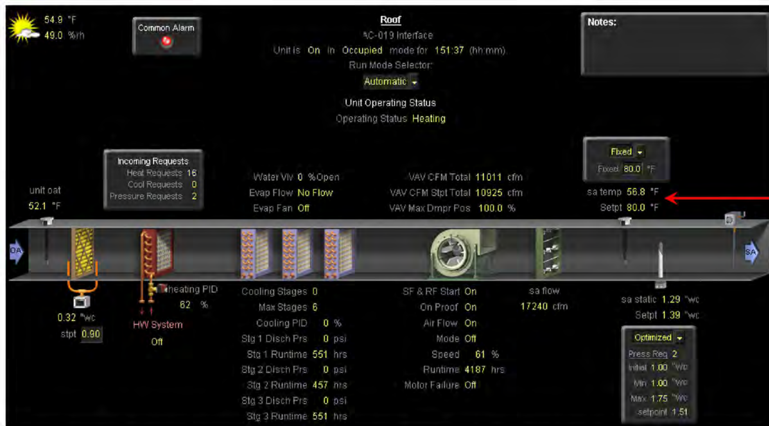
Figure 18: AC-19 supply air temperature in fixed setpoint mode 12 at 4:22 PM, switched back to heating by setting temperature setpoint at 80°F. Cooling section off again, heating valve open to 62%.
