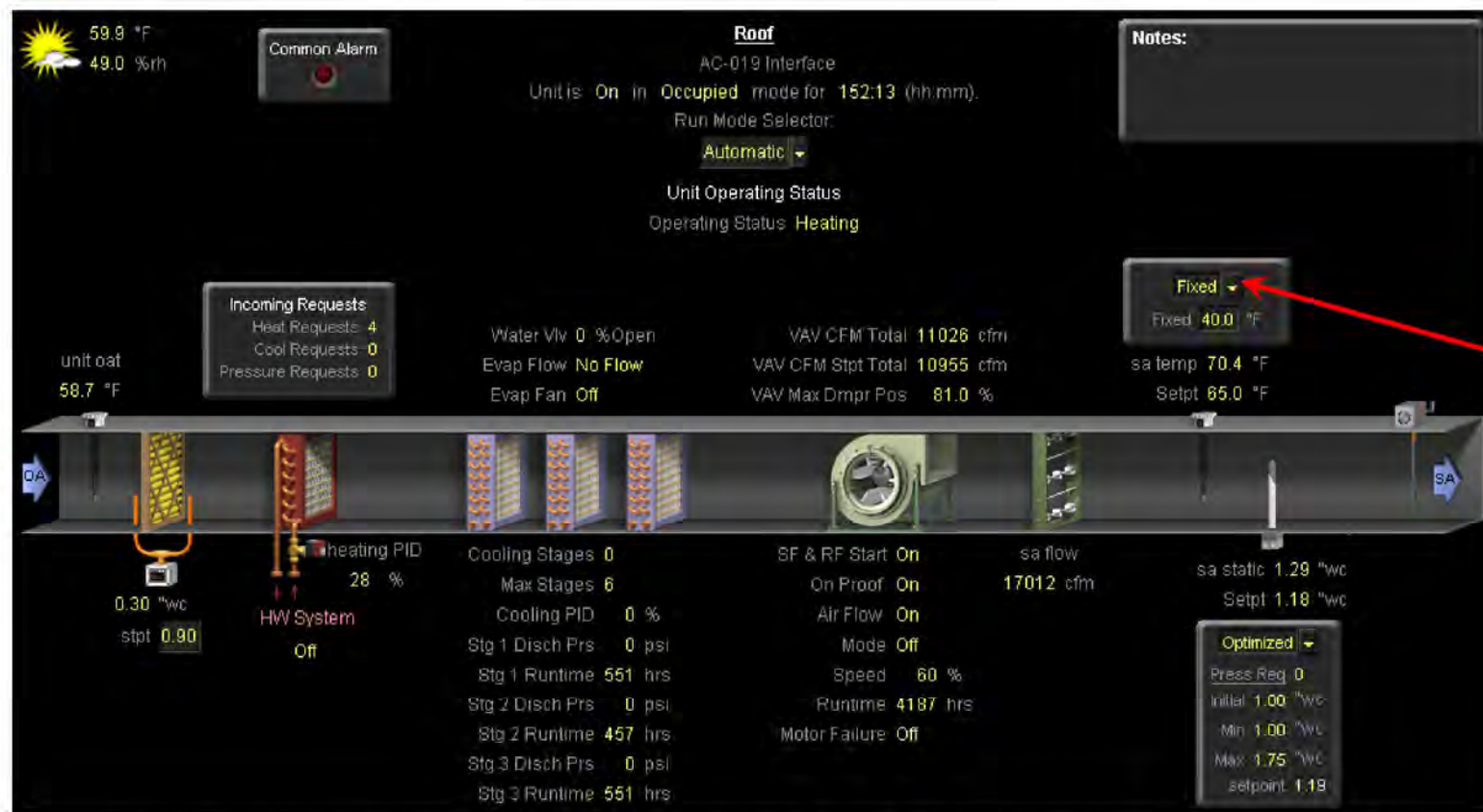
Figure 15: AC-19 supply air temperature in fixed setpoint mode [REDACTED] 12 at 3:47PM, in cooling mode with cooling off.
