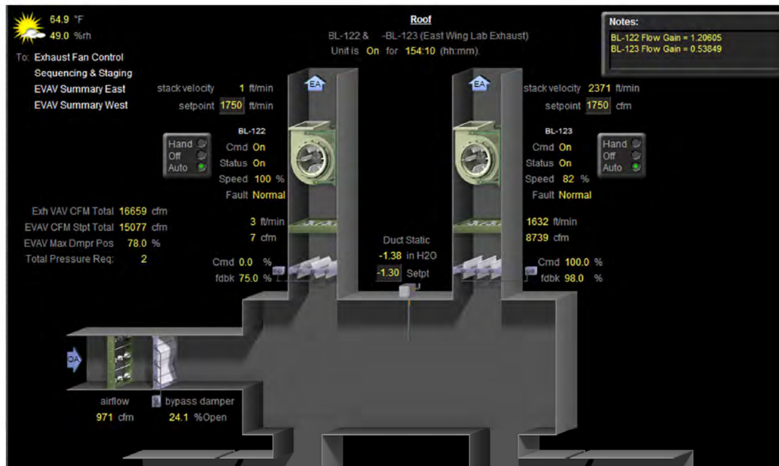
Figure 79: East side exhaust plenum before switch to E –power, 1:47PM. Note that stack velocity sensor for BL-122 is broken, giving an almost zero reading, causing BL-122 to run at full speed
