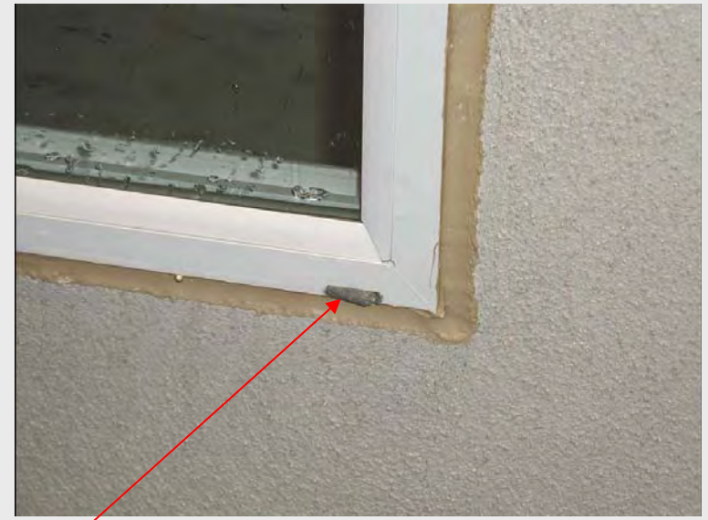
Plugged Weep Holes in Lab to Provide Head Pressure
