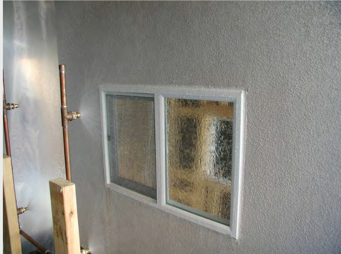
Spray Test on Stucco with Freshly Caulked Window Frames
