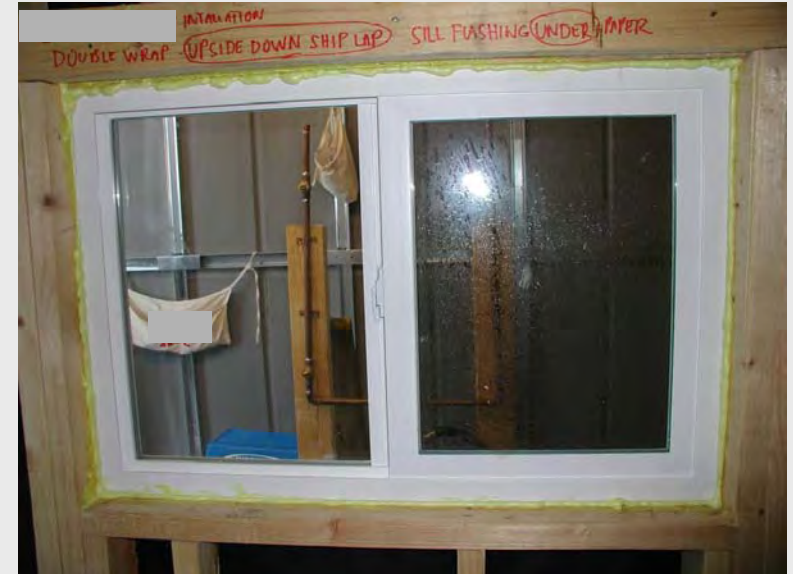
Effective even with reverse shiplap 2-ply building paper
