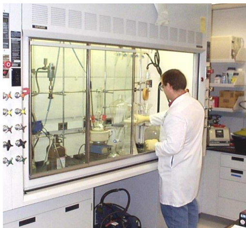
Horizontal Sash Opening
