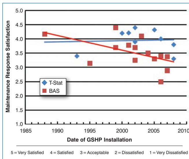
**Figure 1:** Occupant satisfaction with maintenance response vs. GSHP system age.
