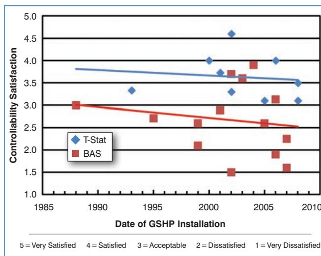
**Figure 2:** Satisfaction with ability to control for thermostat and building automation systems.
