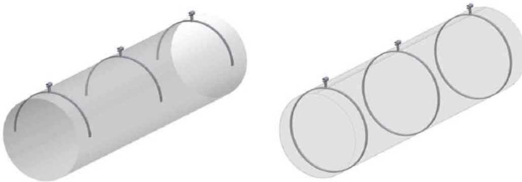
Figure 9-X Inflated internal arc Figure 9-X Hoop system
