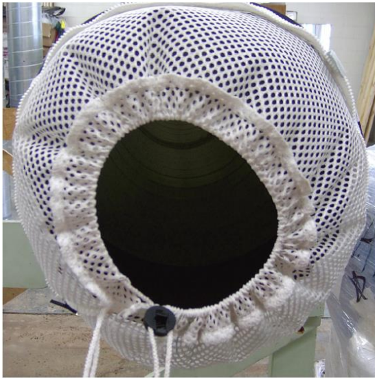
Figure 9-13 Fabric Adjustable Flow Device
