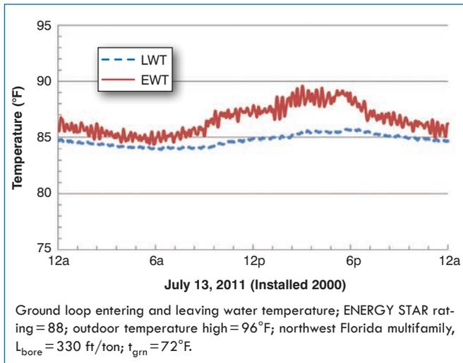
**Figure 3:** Hot day loop temperatures for 78,000 ft<sup>2</sup> (7200 m<sup>2</sup>) Florida apartment complex.
