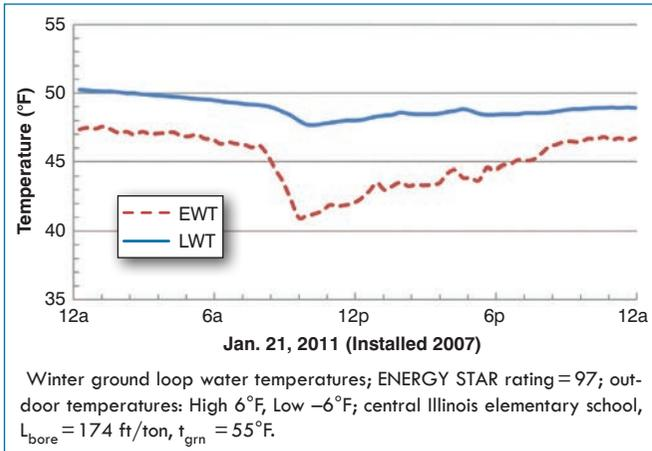
**Figure 12:** Cold day loop temperatures for 37,400 ft<sup>2</sup> (3450 m<sup>2</sup>) central Illinois elementary school.
