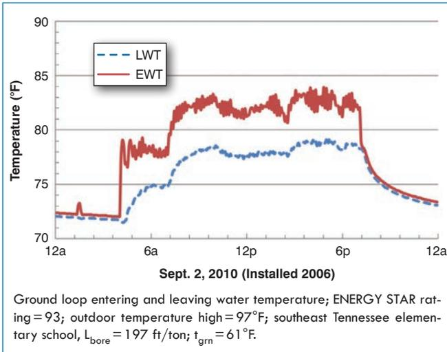
**Figure 1:** Hot day loop temperatures for 70,000 ft<sup>2</sup> (6500 m<sup>2</sup>) Tennessee elementary school.
