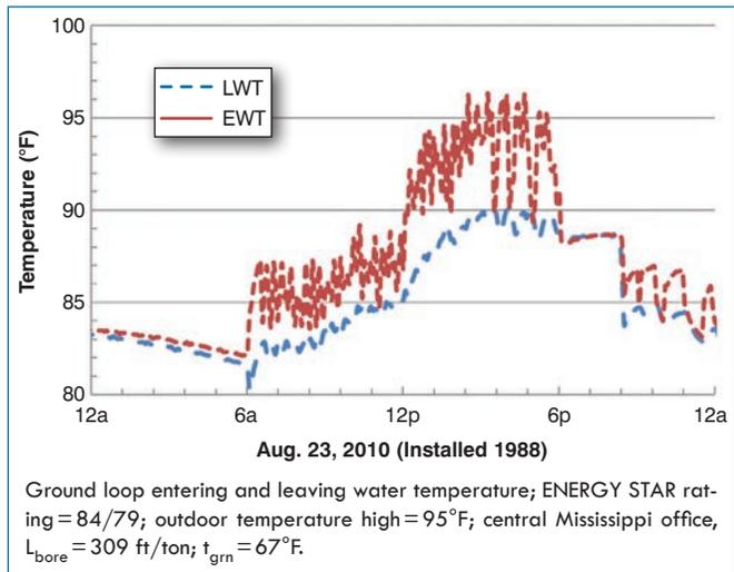
**Figure 4:** Hot day loop temperatures for 5,000 ft<sup>2</sup> (460 m<sup>2</sup>) central Mississippi office.
