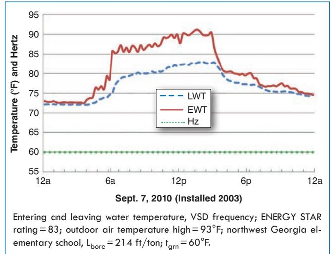
**Figure 2:** Hot day loop temperatures and VSD speed for 85,000 ft<sup>2</sup> (7900 m<sup>2</sup>) Georgia school.
