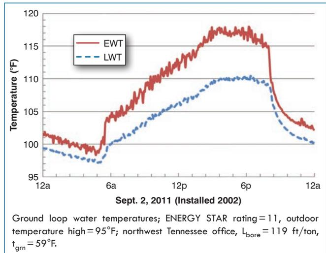
**Figure 11:** Hot day loop temperatures for 37,000 ft<sup>2</sup> (3400 m<sup>2</sup>) northwest Tennessee office.
