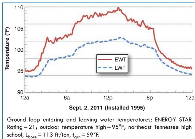
**Figure 9:** Hot day loop temperatures for 161,000 ft<sup>2</sup> (15 000 m<sup>2</sup>) northeast Tennessee high school.
