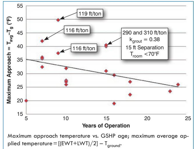
**Figure 13:** Maximum average ground loop-to-ground approach temperatures vs. GSHP age.
