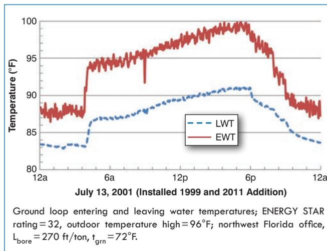
**Figure 6.** Hot day loop temperatures for 59,000 ft<sup>2</sup> (5500 m<sup>2</sup>) northwest Florida office.
