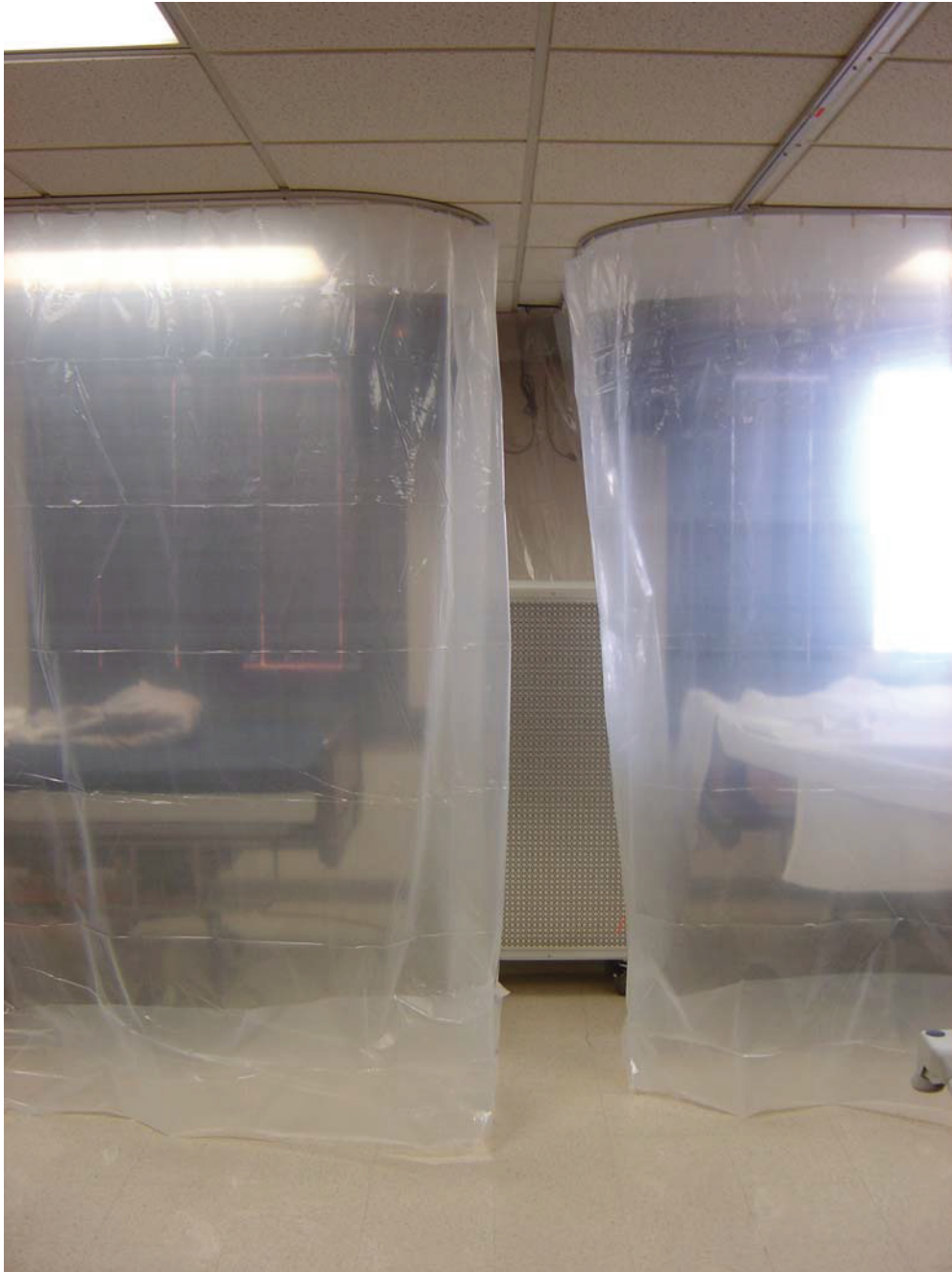
Figure A.3.1 Plastic sheet containment curtains erected around adjacent patient beds in a multiple-patient hospital room. Hem weights had not yet been added. A HEPA-filtered unit exhausted only one unit or both units simultaneously in the experiments, and recirculated filtered air to the room.
