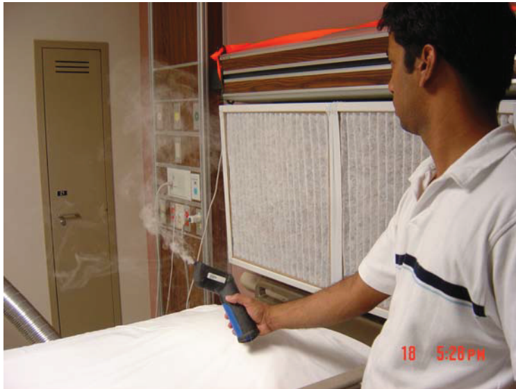
Figure A.2.3 Qualitative capture test using neutrally buoyant mist showing failure to provide directed air flow.
