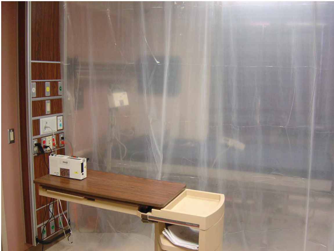
Figure A.3.2 A 10-inch opening in the curtain near the head of the patient bed allowed some directional airflow to be established diagonally across the patient and toward the HEPA unit at the foot end of the bed. Also shown in the photo are three of the Grimm aerosol spectrometers – one on the bed and one at provider nose height inside the enclosure, and one on the meal tray table outside the enclosure.
