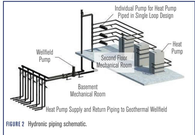
FIGURE 2 Hydronic piping schematic.
